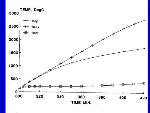
Figure 7 Heat Up of Core Debris in CANDU 6 Calandria, Reference Conditions
